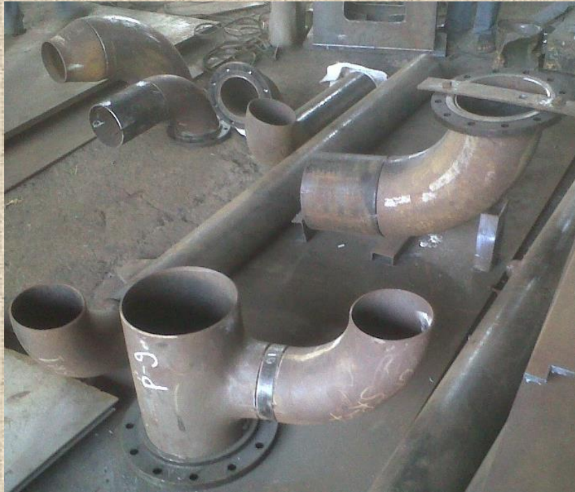
BURNER SYSTEM PIPING SPOOL FOR L&T AEROSPACE
