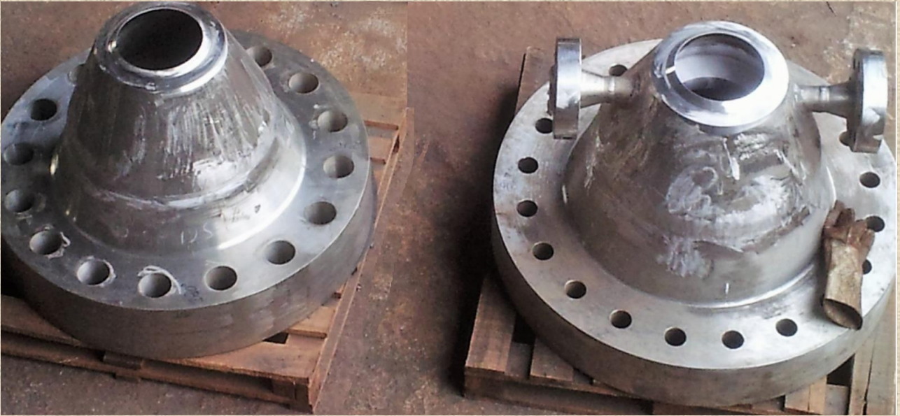
46MM THICK SS304L EXPANDER AND REDUCER ASSLY WITH 200MM THICK FLANGE FOR L&T AEROSPACE
