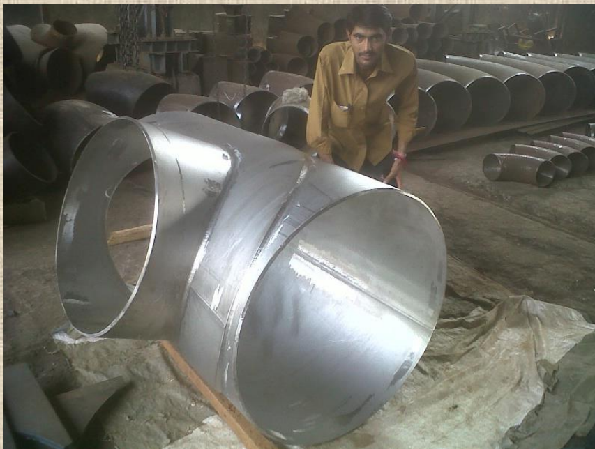
BRANCH WELDED SS316L TEE WITH RF PAD, DESIGNED & MANUFACTURED AS PER ASME B31.3
